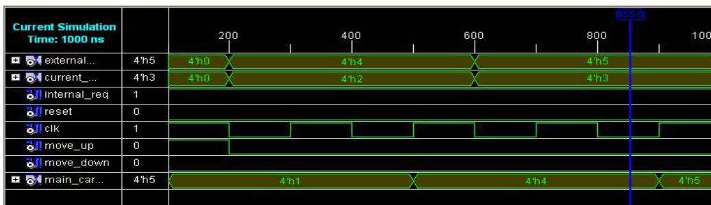
Figure 3.6 Simulation result of selective-up algorithm
