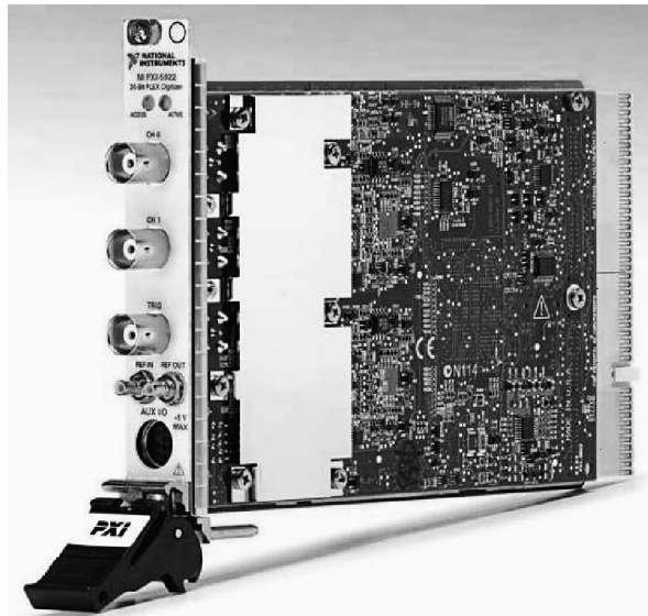
Figure 16.41 Instrument function on a PC card. Photo courtesy of National Instruments Corporation.
