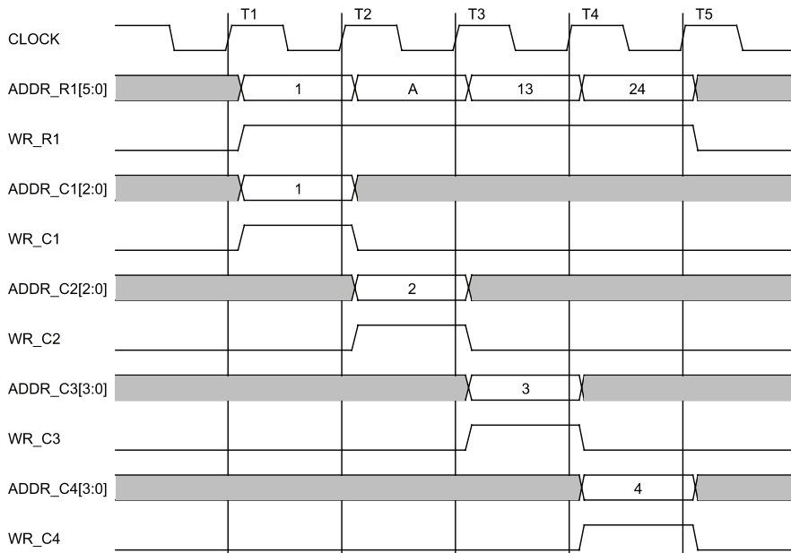
Figure 4.34 Address-translation waveform for a decoding-friendly address map
