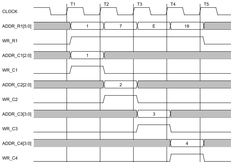
Figure 4.30 Interconnect address translation with a tightly packed address map
