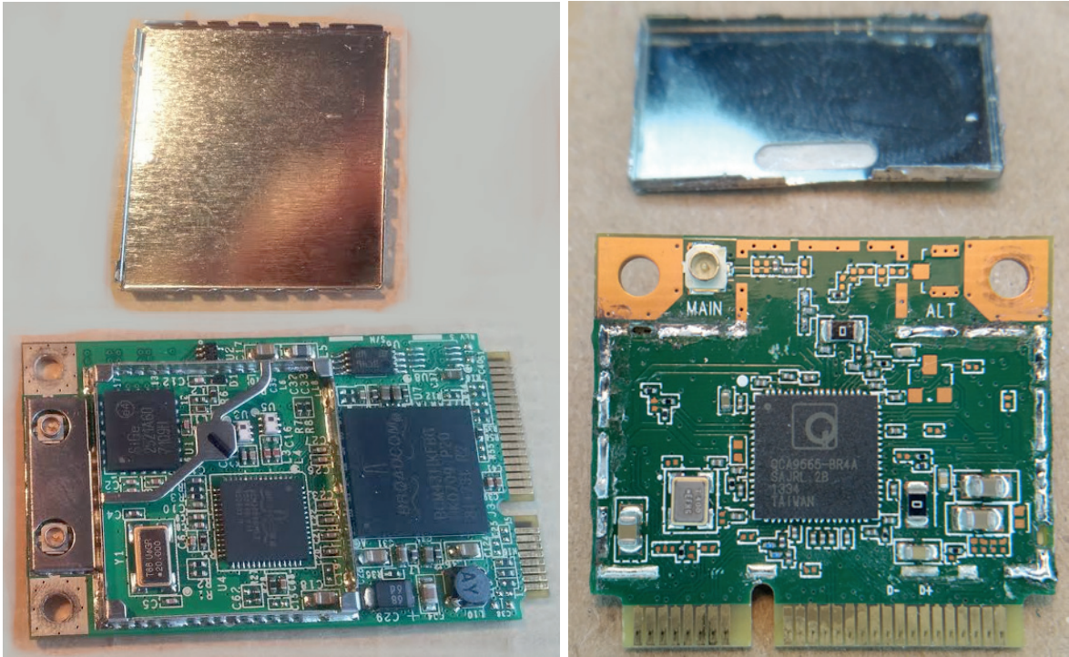
Figure 6.3 Two PCIe 802.11 Wi-Fi modules for a laptop. Their shielding lids have been removed. The older unit, on the left, has a three-chip set from Broadcom. It is physically nearly twice the size of the newer unit, shown on the right, which has been magnified 2×. The new unit uses a Qualcomm QCA9565 device that has a higher throughput and also includes Bluetooth. The only other active part needed is the 40-MHz crystal oscillator to the left of the chip. As can be seen at top right, to give a lower-cost lower-performance product, the second of the two diversity antenna sockets, labelled 'ALT', was not fitted
