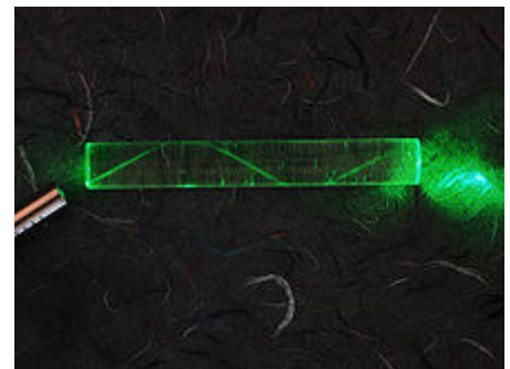
A laser bouncing down an acrylic rod, illustrating the total internal reflection of light in a multi-mode optical fiber.
