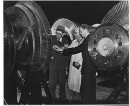
Belgian electrical engineers inspecting the rotor of a 40,000 kilowatt turbine of the General Electric Company in New York City
