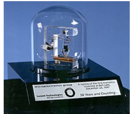
A replica of the first working transistor, a point-contact transistor.
