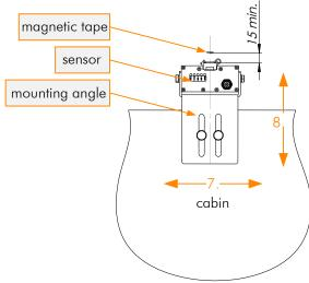
8. Adjust now the distance between sensor and band. Up to a travel height of 50m we recommend an offset of at least 15 mm. This will ensure steady contact between steel side of the band and the polymer guide of the sensor.
