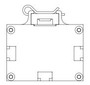
Illustration1: Mounting notches on sensor
