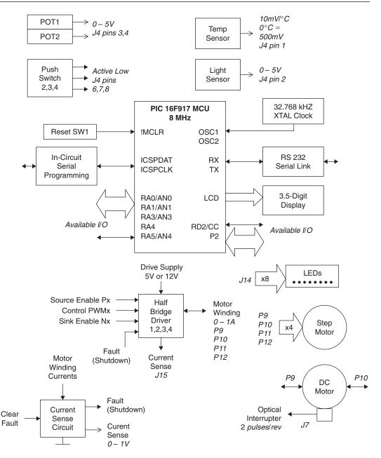
Figure 4.2: Block Diagram of PICDEM Mechatronics Board
