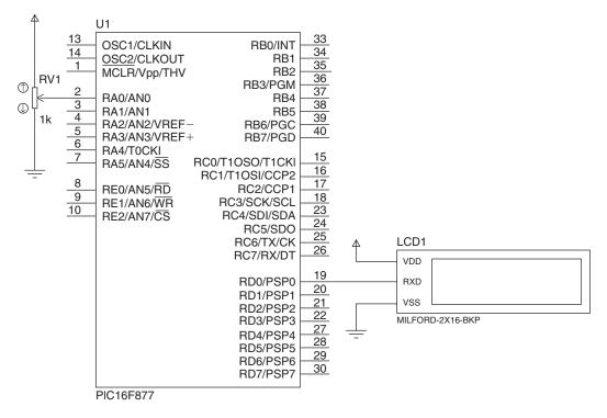
Figure 3.1: Single Analog Input and Display Test Circuit
