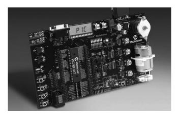
Figure 4.1: PICDEM Mechatronics Board (by permission of Microchip Inc.)
