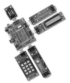
Figure D.2: Matrix Multimedia Modular PIC System
