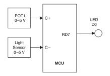
Figure 4.11: Comparator Test Setup
