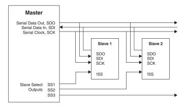
Figure 1.12: SPI Connections
