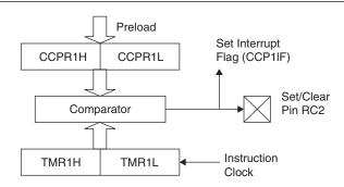
Figure 3.4: Compare Hardware Block Diagram
