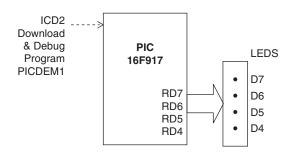
Figure 4.5: Block Diagram of Test Hardware Configuration
