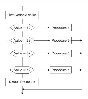
Figure 2.10: Switch..Case Branching Structure
