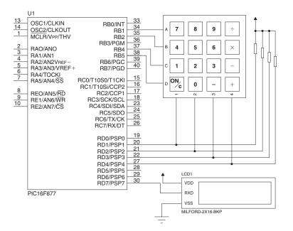
Figure 2.12: Calculator Schematic
