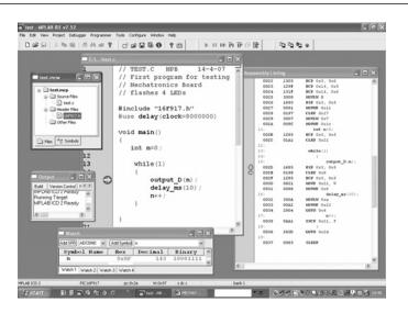
Figure 4.6: Test Program Debugging Screen
