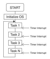
Figure 5.7: Basic RTOS Operation
