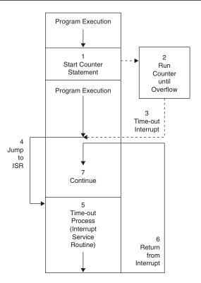
**Figure 1.9: Timer Interrupt Process**
