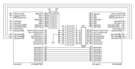
Figure 3.10: PSP Test System
