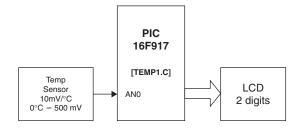
Figure 4.12: Temperature Sensor System
