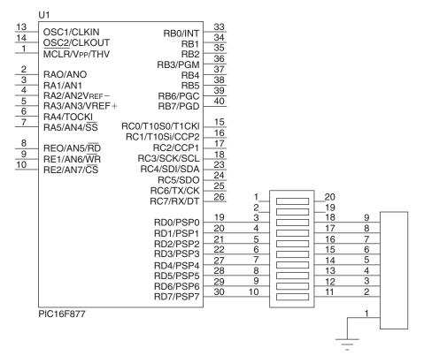
Figure 2.2: OUTBYTE Test Circuit with Output LEDs
