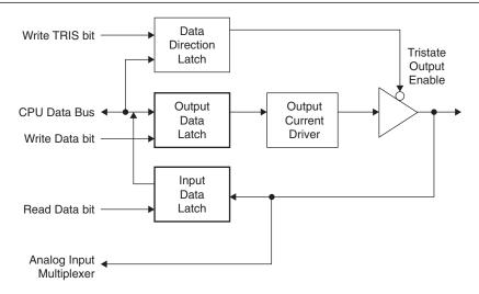
Figure 1.4: I/O Pin Operation
