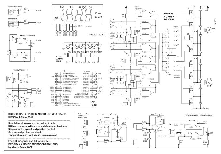
Figure 4.14: PICDEM Mechatronics Board Simulation Schematic
