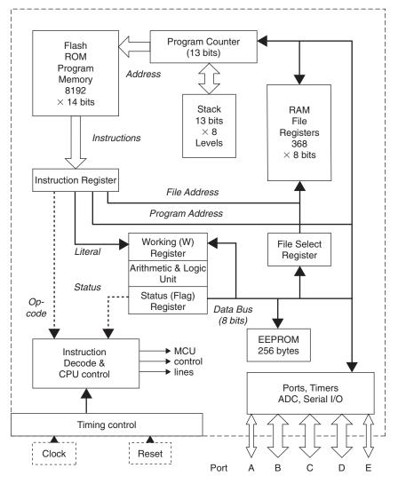
Figure 1.3: PIC16F877 MCU Block Diagram
