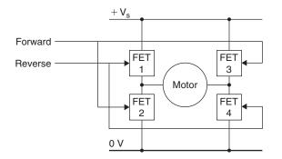
Figure 4.4: Full-Bridge Driver Connection of the DC Motor
