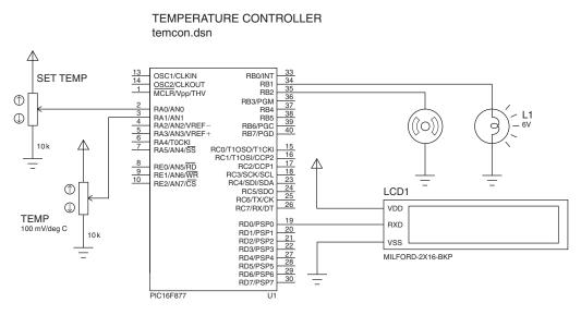
Figure 5.2: Temperature Control System
