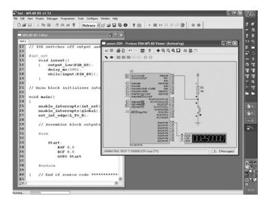
Figure 2.15: Debug Screenshot of FAST.C Showing Output Frequency
