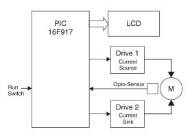
Figure 4.8: Block Diagram of Motor Test System
