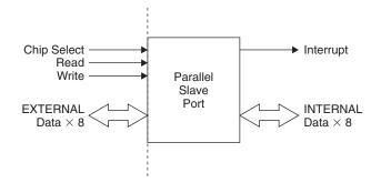
Figure 1.8: Parallel Slave Port Operation
