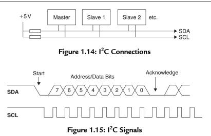
The sequence to read a single byte requires a total of 5 bytes to complete the process, 3 to set the address, and 2 to return the data. Thus, a substantial software overhead is involved. To alleviate this problem, data can be transferred in continuous blocks (memory page read/write), which speeds up the transmission.
