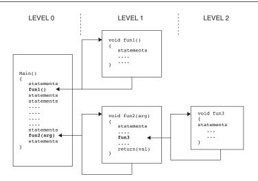
Figure 2.11: Hierarchical C Program Structure
