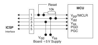
Figure 1.18: ICSP Target Board Connections
