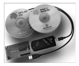
Figure 1.17: PICkit2 Demo System Hardware (reproduced by permission of Microchip Inc.)
