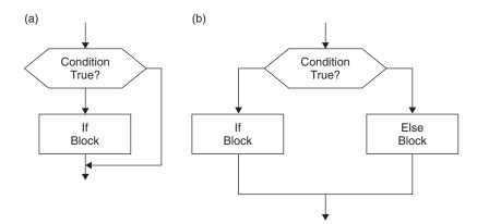
Figure 2.9: Comparison of (a) If and (b) If .. Else
