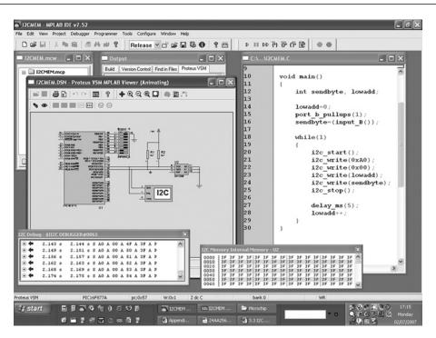
Figure 3.9: I<sup>2</sup>C Test System
