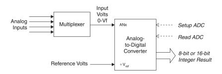
Figure 1.6: ADC Operation
