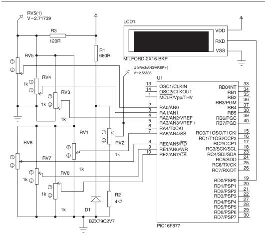
Figure 3.2: Input Voltage Measurement and Display
