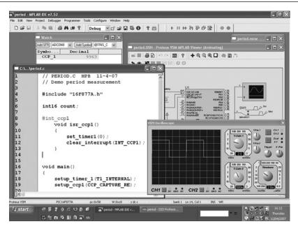
Figure 3.6: Capture Mode Used to Measure Input Period
