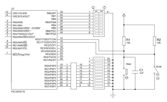
Figure 3.11: EEPROM Test System
