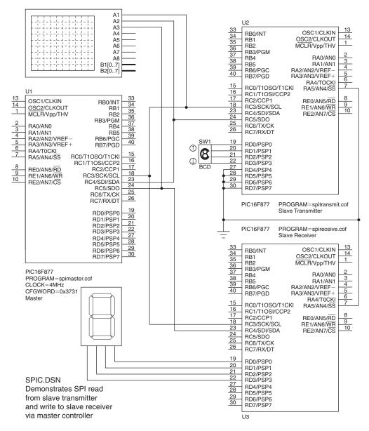
Figure 3.8: SPI Test System Schematic
