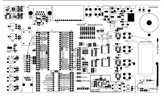
Figure 4.3: Mechatronics Board Layout (by permission of Microchip Inc.)
