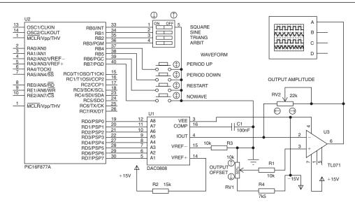
Figure 3.12: Waveform Generator
