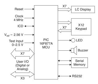
Figure 5.3: BASE Board Block Diagram
