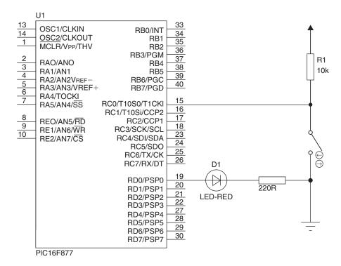
Figure 2.4: INBIT.DSN Test Circuit with Input Switch
