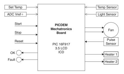
Figure 4.13: Block Diagram of the Temperature Controller
