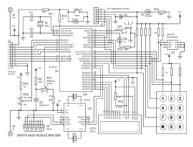
Figure 5.4: BASE Board Circuit Diagram
