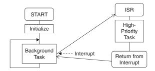
Figure 5.6: Basic Interrupt Operation
