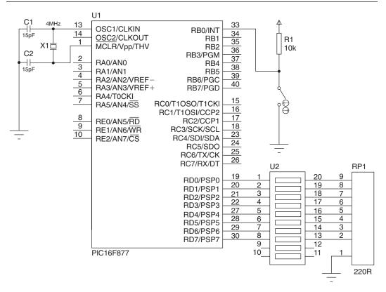
Figure 3.3: External Interrupt Test Hardware
