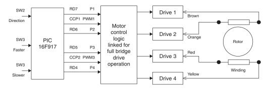
Figure 4.10: Stepper Motor Test System Connections
