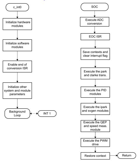
Figure 7-2. System Software Flowchart
