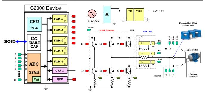
Figure 7-1. A 3-Phase Induction Motor Drive Implementation
