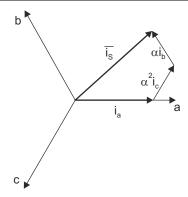
Figure 4-2. Stator Current Space Vector and Its Component in (a,b,c)
