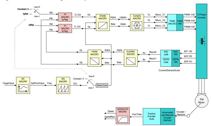
Figure 9-11. Level 3 - Incremental System Build Block Diagram
