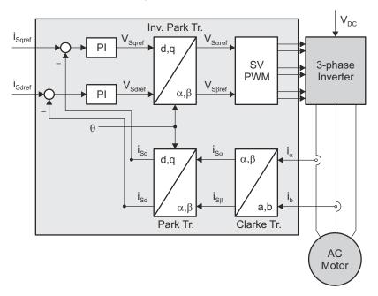
Figure 5-1. Basic Scheme of FOC for AC Motor
