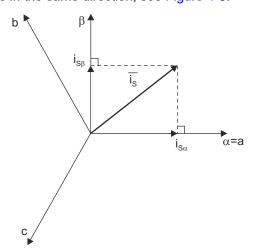
Figure 4-3. Stator Current Space Vector and Its Components in the Stationary Reference Frame
