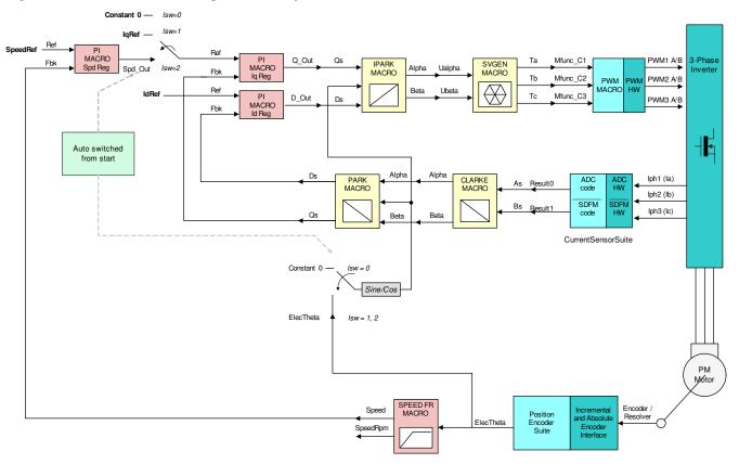
Figure 9-13. Level 4 - Incremental System Build Block Diagram
