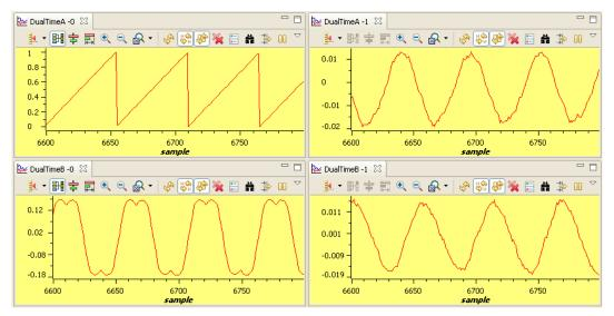
Figure 9-14. Measured theta, sygen Duty Cycle and Phase A and B Current Waveforms Under No-Load and 0.3 pu Speed
