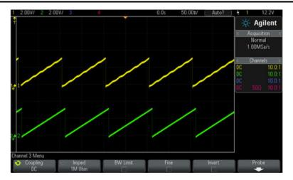
Figure 9-9. Scope Plot of Reference Angle and Rotor Position
