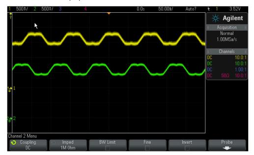
Figure 9-3. DAC 1-4 Outputs Showing Ta, Tb Waveforms
