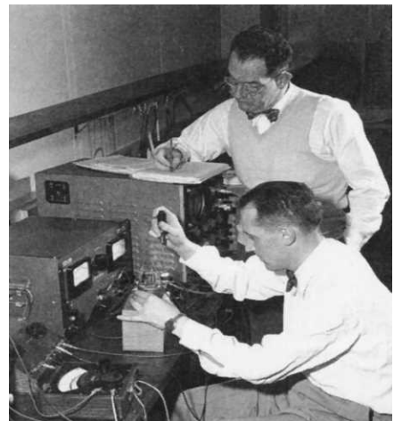
(b) Drs. Ian Munro Ross (front) and G. C. Dacey jointly developed an experimental procedure for measuring the characteristics of a FET in 1955.
