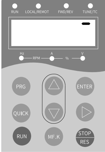
Figure 12-4 Light curtain signal valid display (segment A)
